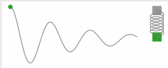
Damped harmonic oscillator
